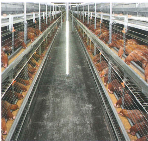
Natura60: perfectly approachable system with a worldwide unique feature: every second inspection aisle remains free of litter, hens and manure.
