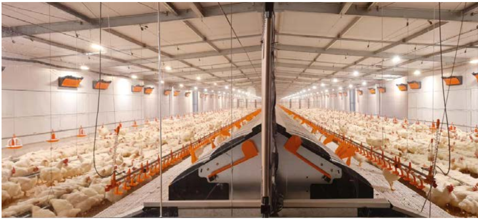
View of a broiler breeder house during feeding: suspended chain feeding system
